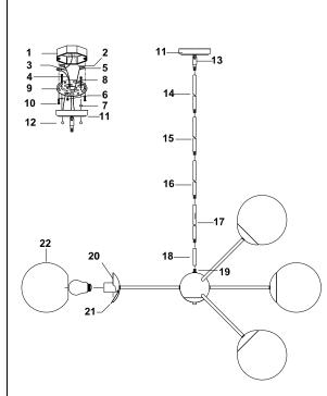
**1. OUTLET BOX** 2. WHITE WIRE **3. BLACK WIRE** 4. GROUND WIRE 5. WIRE CONNECTOR 6. GROUND SCREW 7. HEX NUT 8. MACHINE SCREW 9. MOUNTING BAR **10. MOUNTING SCREW** 11. CANOPY 12 BALL NUT 13. SWIVEL 14. STEM (L12") 15. STEM (L12") 16. STEM (L12") 17 .STEM (L6") 18. STEM (L3") **19. FIXTURE FRAME** 20. SOCKET CUP 21. SPRING CLIP 22. GLASS
